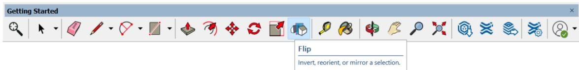
Like several other tools, you can activate Flip after selecting geometry or hover over the entities you want to flip. Once engaged, you'll see three planes corresponding to the model's orientation. Hover over a plane and click once to 'flip' about that plane. You can even use the arrow keys - left arrow for green, right arrow for red, and up for blue.
